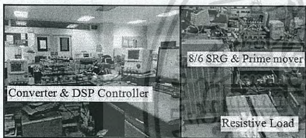
(b) Converter and a TMS320F2812 DSP Controller, Prime mover and the SRG, and Resistive load
