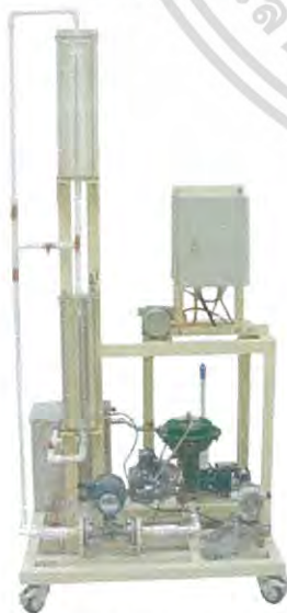
Fig. 2. FF-based level-control plant model employed in experiments.
