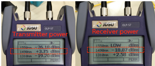
Fig. 6. Optical power testing with PON optical power meter
