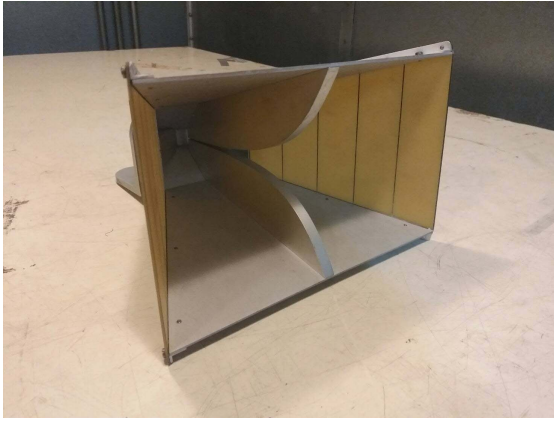
Fig. 3. Double-ridged waveguide horn antenna.
