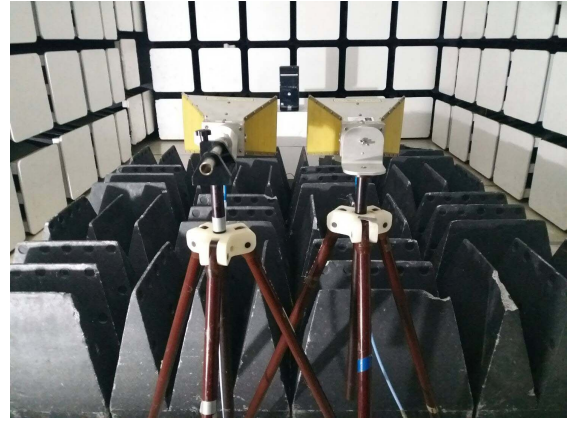
Fig. 4. Measurement setup for monostatic radar channel.
