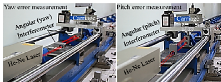
Fig. 6. Yaw and pitch error measurement using a laser interferometer.
