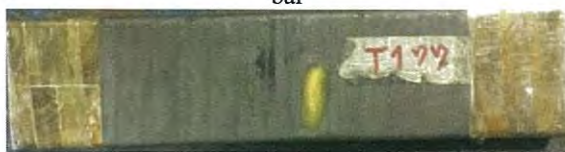
Fig.4. Degradation from partial discharge
