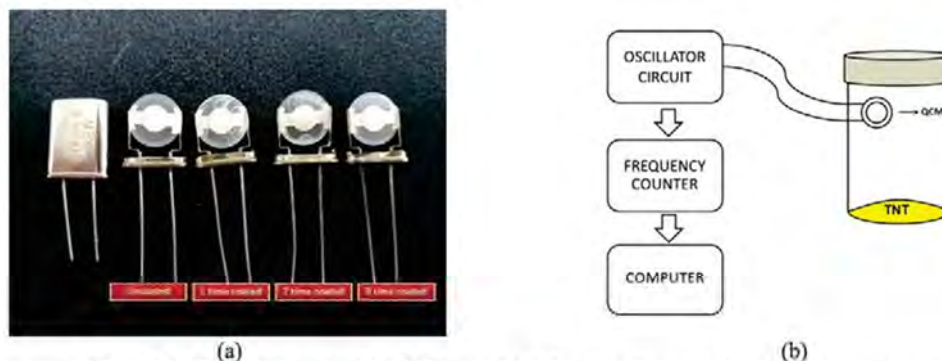
FIGURE 2. The photograph of (a) QCM and (b) Schematic diagram of system for measurement
