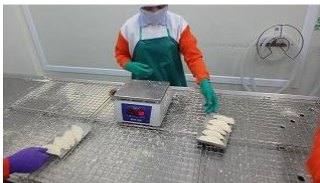
Figure 4.5 Workstation 6 after improvement, check weight of product
