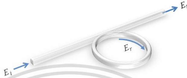
Figure 3.6 Schematic diagram for a ring resonator coupled to a single waveguide
