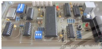
Fig. 7. Photograph of digital signal control (DSC) and dead time circuit board
