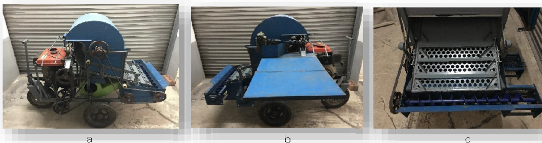
Figure 2 (a) Groundnut Stripping Machine (b) Feeding Tray (c) Sieve and Screw Convey
