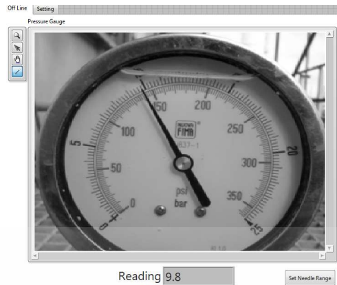
Figure 10 Front panel and show result by using Lab view
