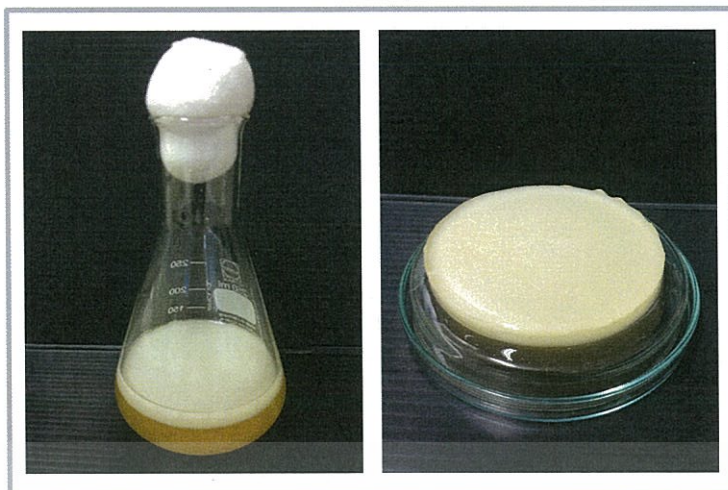
Figure 2.3 BC pellicle produces in static culture.
