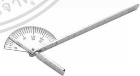
Fig. 4. Baseline finger (small joint) goniometer.
