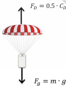
Fig.3. The two forces acting on the CanSat.
