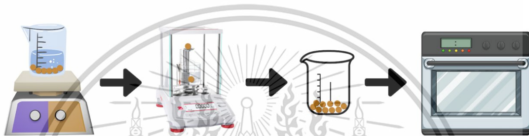
Figure 3.5. Archimedes method to analyze physical properties of fired-clay balls.
