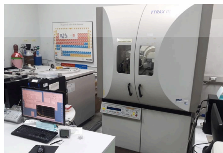
Figure. 3.10 The XRD diffractometer (Rigaku, TTRAX III) at MTEC. This material is reserved for educational use only, not allowed for commercial use.
