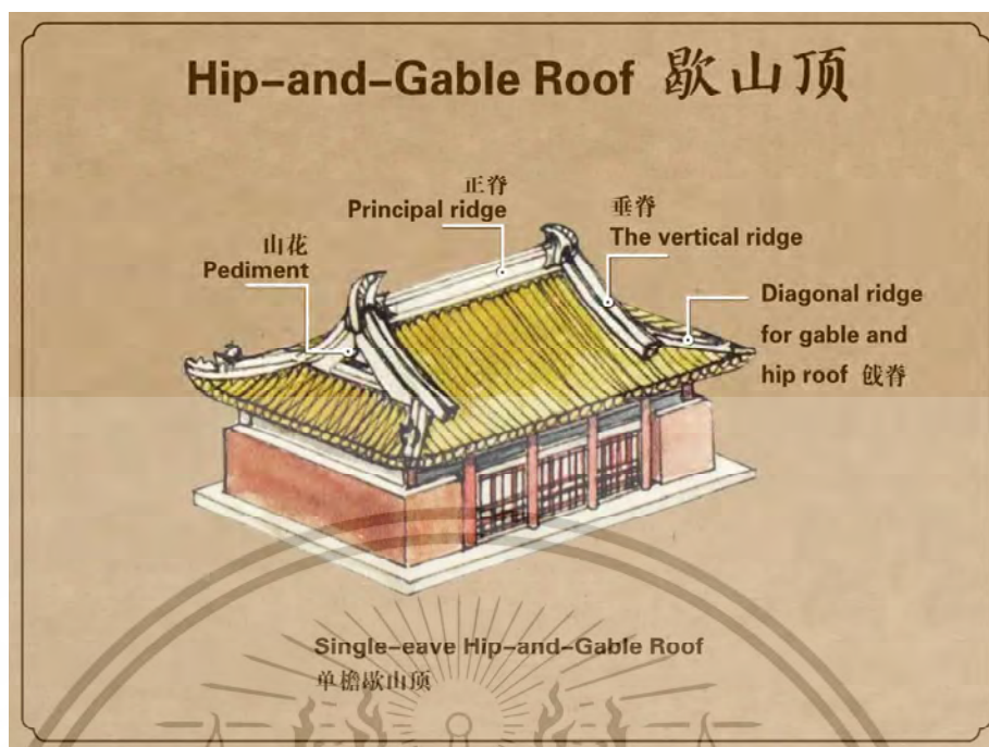
Figure 4.6 Introduction to the Form of Hip-and-Gable Roof
