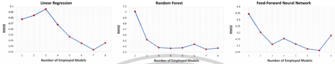
FIGURE 8. Incremental performance improvement in level-1 models. This figure illustrates RMSE progression for Level-1 models predicting CPU requests (unit: percent), highlighting the incremental performance enhancements achieved with each addition of a Level-0 model.
