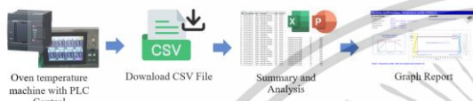
Figure 2 shows the manual process of downloading oven temperature data and creating a report for the Image Sensor product
