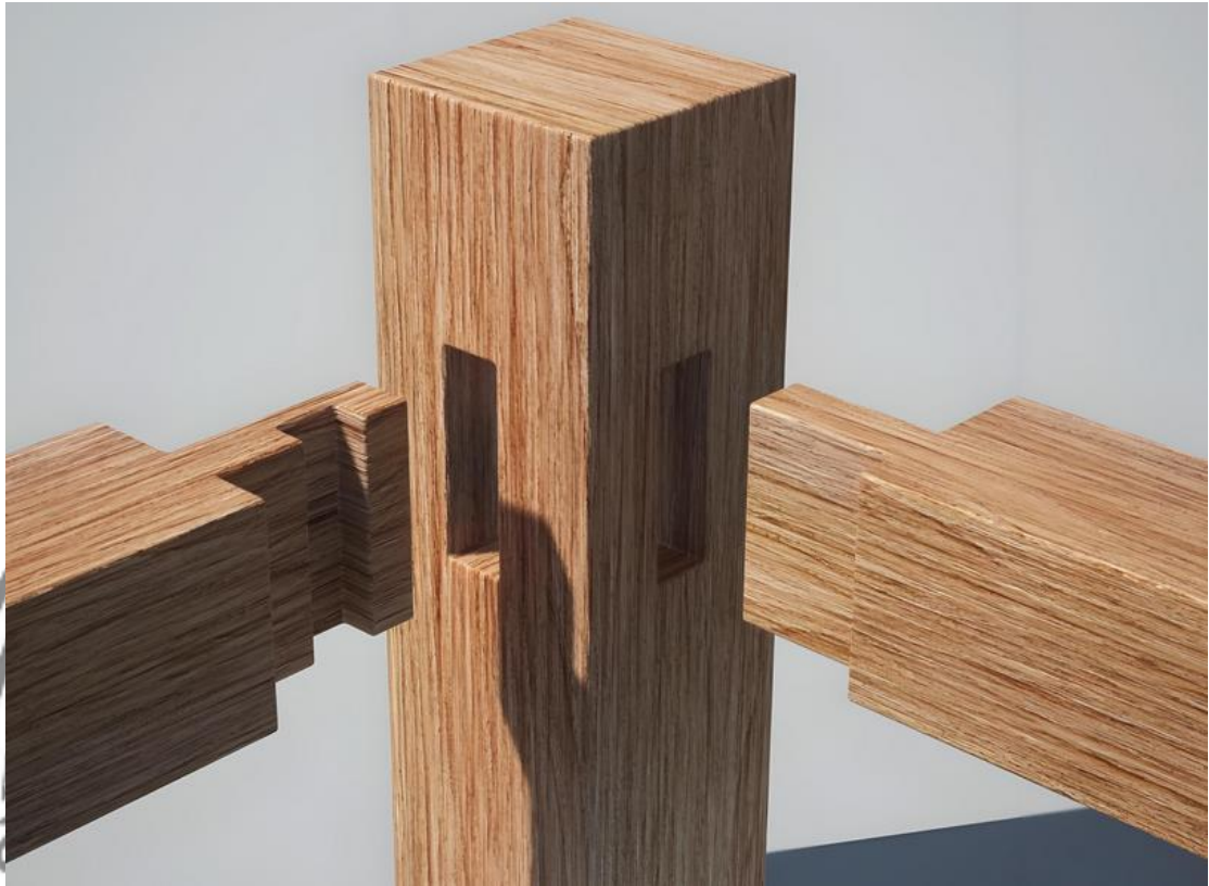
Figure 4.23 Mortise and tenon structure diagram Source: www.baidu.com
