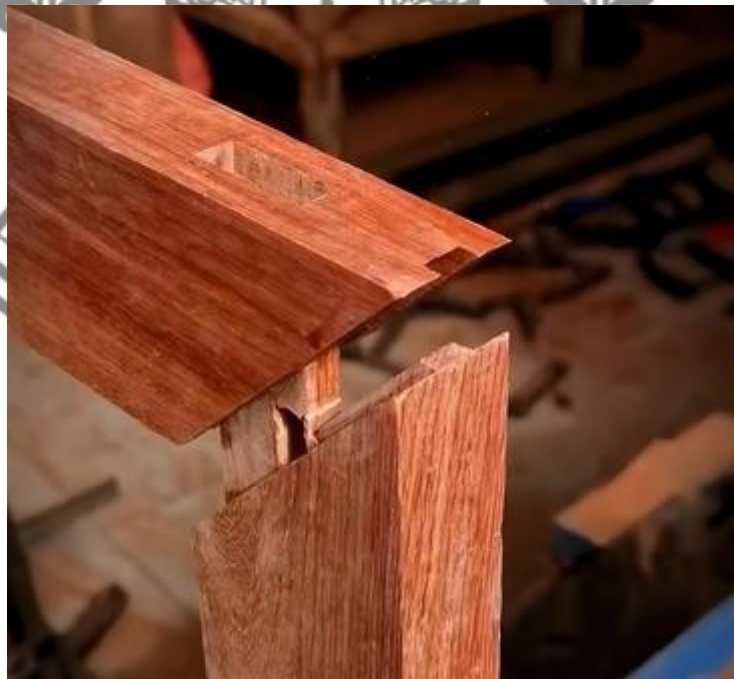
Figure 4.24 Mortise and tenon structure link Source: www.baidu.com
