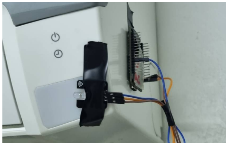
Figure 3.31 Air Conditioner Controller
