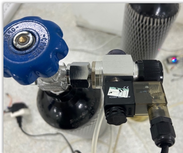
Figure 3.30 Carbon Dioxide Controller
