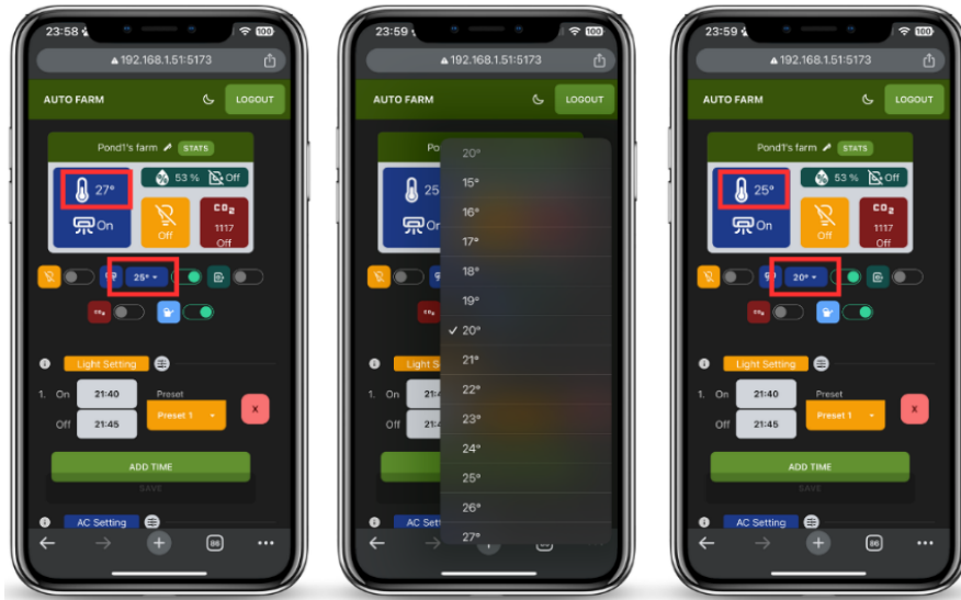
Figure 4.10 Changing the temperature of the air conditioner.
