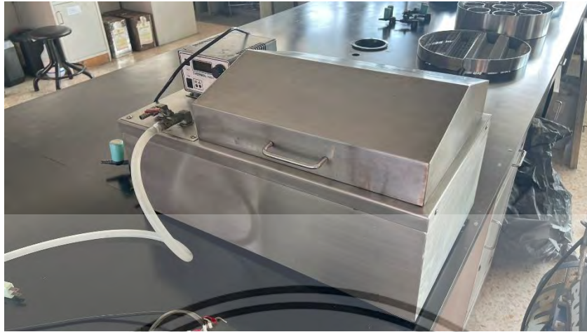
Figure B1-7 Saltwater tank
