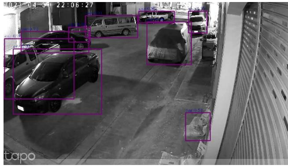
Figure 33 NIGHT detection with grayscale
