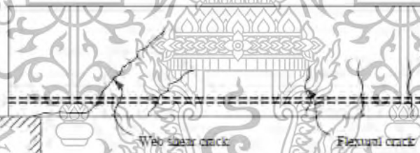
Figure 14: Web shear crack [10]
