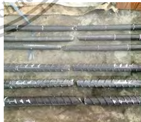
Figure 30 : After testing the steel specimen
