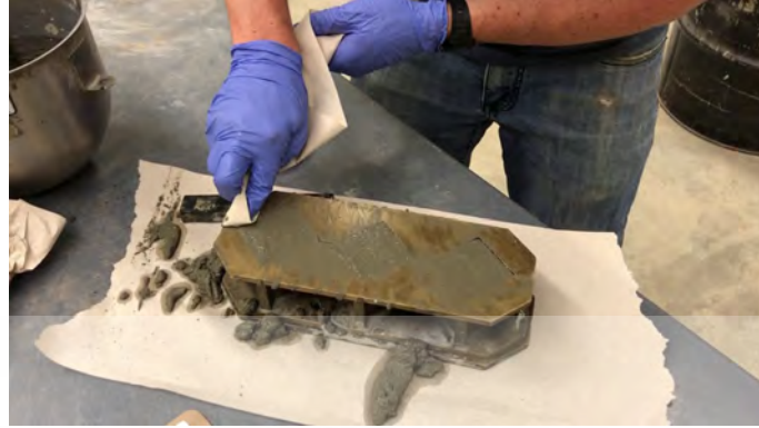
Figure 22 : Casting concrete specimen cube shape.
