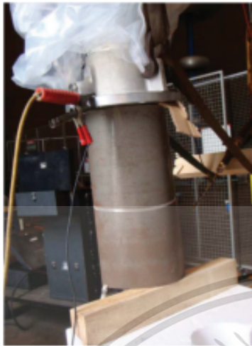
Fig. 4. The extended diameter of the bottom part of the bushing with the sheet metal.
