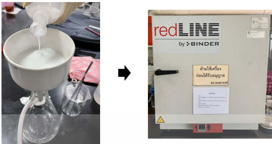
Figure A-6. Separate obtained zeolite NaA and solution using Buchner repeat this step until pH < 9. After separation, put Zeolite NaA into oven at 110 °C for 24 hr.
