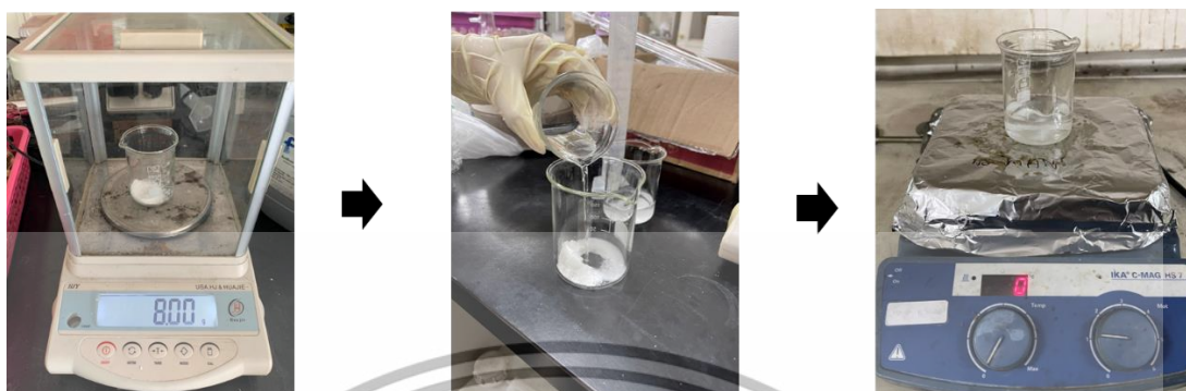
Figure A-1. Dissolve 13.89 g of sodium metasilicate pentahydrate with 37.17 g of deionized water using a magnetic stir to the homogenous liquid mixture.
