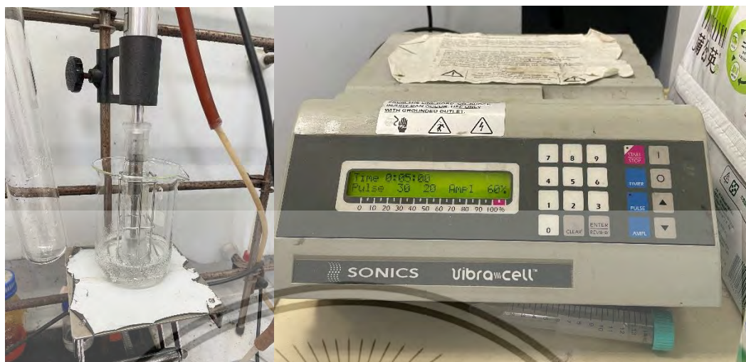
Figure 12. Setup for probe sonicator and setting for Timer, Pulse and amplitude
