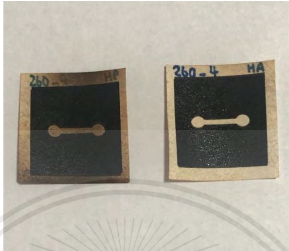
Figure 4-3. The comparison of the color paper which influence from the heater between heating on the hotplate (Left: 1 hour at 260 °C) and heating in the hot air oven (Right: 15 minutes at 260 °C)
