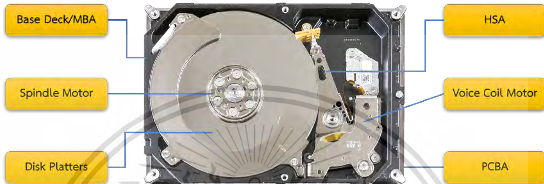
Figure 2.1 Hard disk drive components
