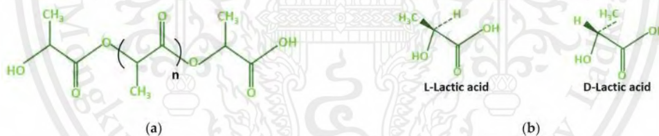
Figure 2. D-content and L-content in Polylactic acid [6]
