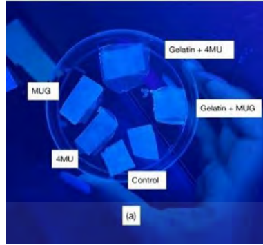
Figure 30. Fluorescence product from the film with pH 3
