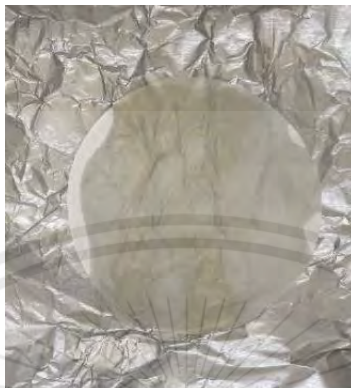
Figure 29. PLA synthesis after annealed was sticky and could not remove from paper
