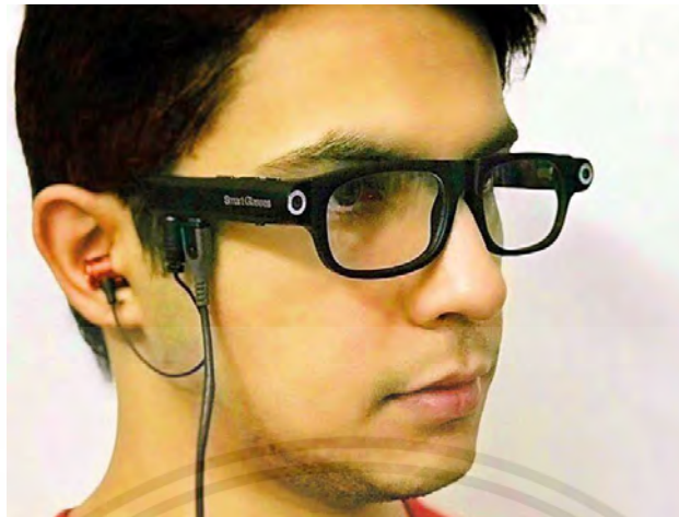
Figure 2.3.3: Example of Smart Glasses for people who are blind and Partially Sighted [7]
