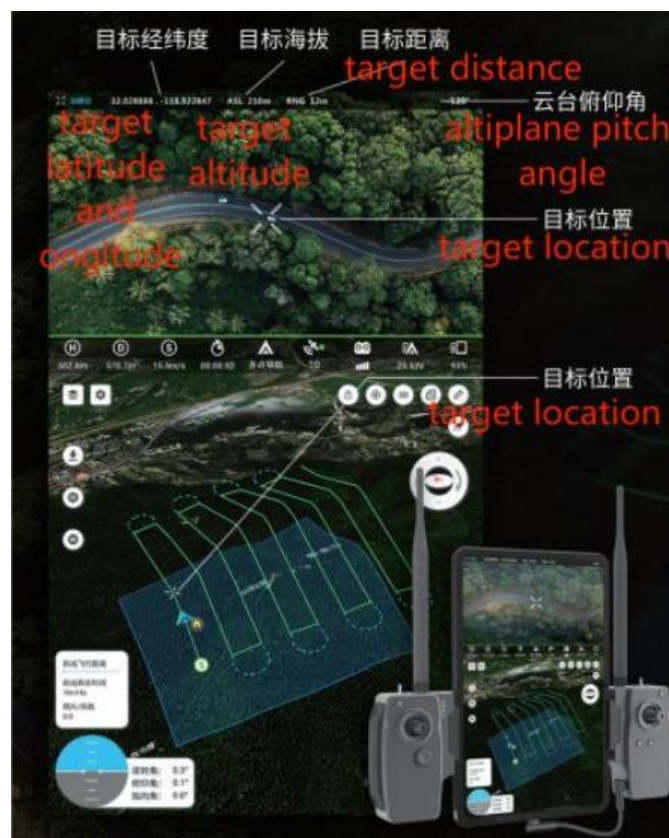
Fig 3-11 HuaCe V200 ground control system
