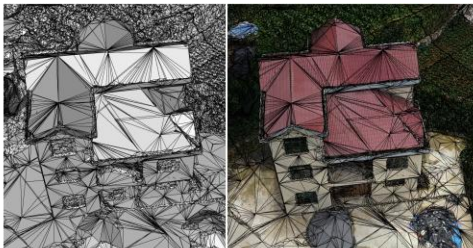
Fig 3-7 Schematic of the effect of TIN triangular mesh with texture mapping
