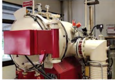
Figure 3-10 High vacuum sintering furnace SCHMETZ D59708 MENDEN
