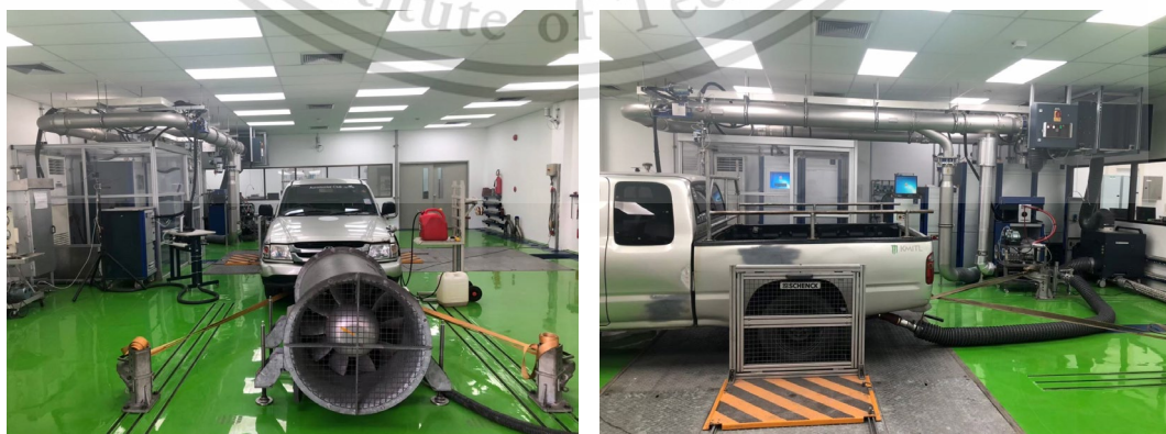
Figure 3.8 Schematic diagram and experimental setup for the regulated emission testing under the new European driving cycle (NEDC)
