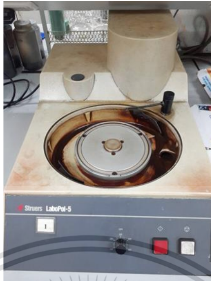
Figure 3. 17 Grinding and polishing of metallurgical machine.
