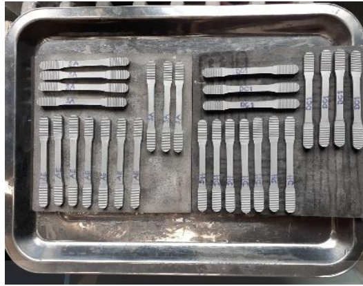
Figure 3. 28 The MPIF standard 10, ASTM B783 standard tensile test bar
