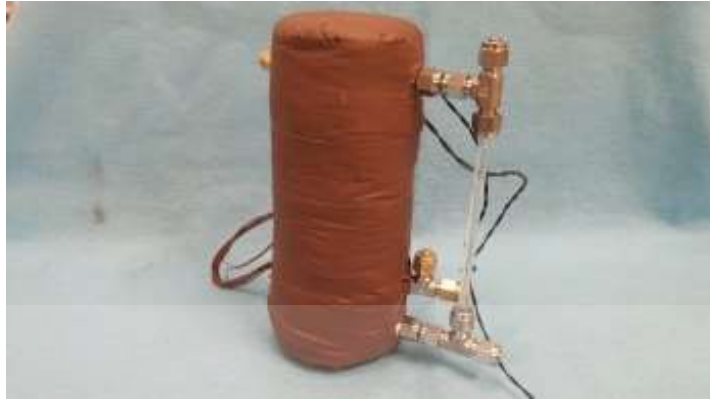
Figure 3.4 Humidification bottle from Fuel Cell Technologies, Inc.
