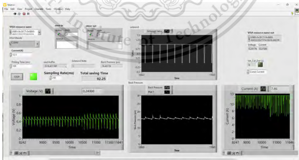
Figure 4.3 LabVIEW HMI of the test system
