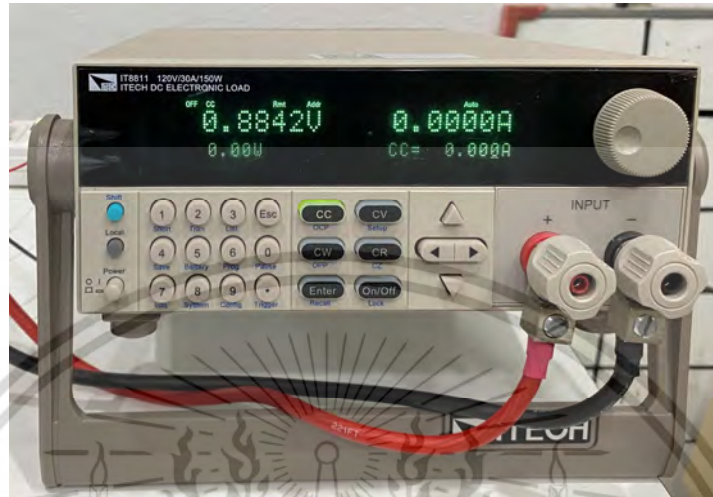
Figure 3.10 High Power DC Electronic Load from ITECH Electronics
