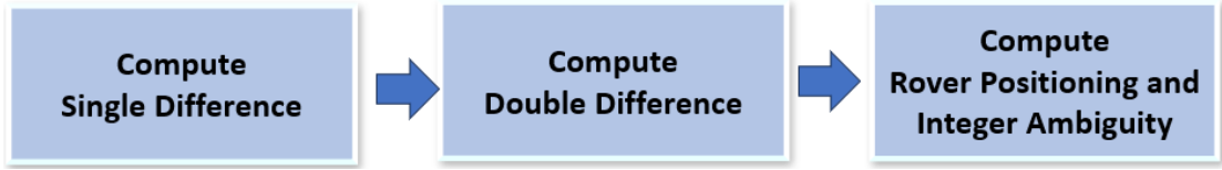
Figure 2.13 RTK positioning procedure for rover's positioning computation
