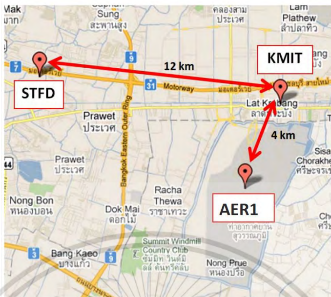
Figure 3.4 Illustrations of the GNSS stations to compute the ionospheric delay gradients near Suvarnabhumi international airport
