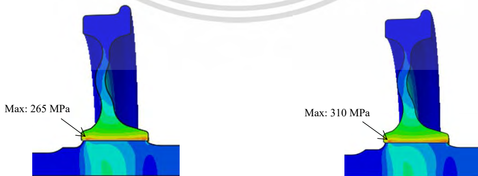
(a) von Mises stress distribution for \delta 240 \mu\text{m} . (b) von Mises stress distribution for \delta 280 \mu\text{m} .
