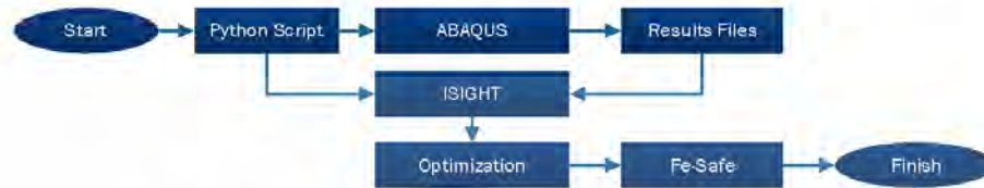
Figure 2. Structural analysis and optimization process workflows chart
