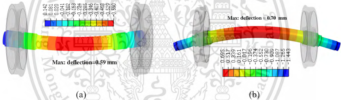
Figure 8.3 Comparison the deflection of the axle under the loading (a) for the assembled inside axle boxes (b) for the assembled outside axle boxes.
