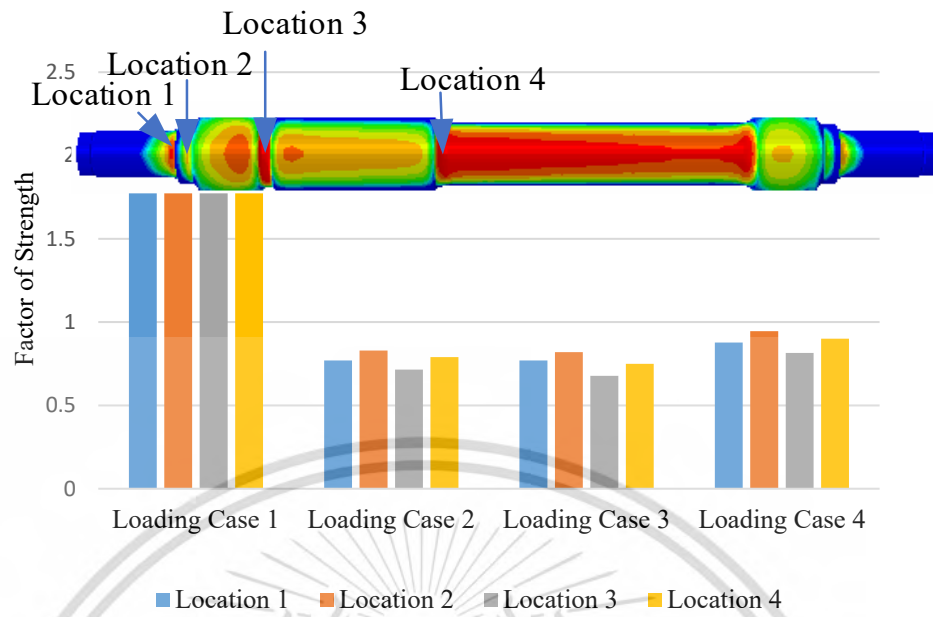
Figure 6.17 Estimated factor of strength of railway axle
