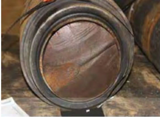
Figure 2.6 Mating fracture surface from the broken axle at the L1 bearing (view toward end of axle) [7]
