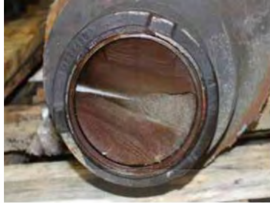
Figure 2.7 Mating fracture surface from the broken axle at the L1 bearing (view toward centre of axle) [7]
