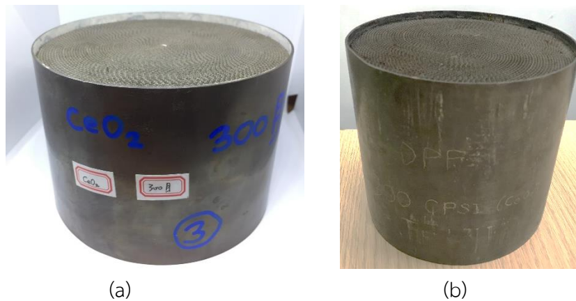
Figure 3-12 (a) Diesel oxidation catalyst and (b) Partial-flow diesel particulate filter
