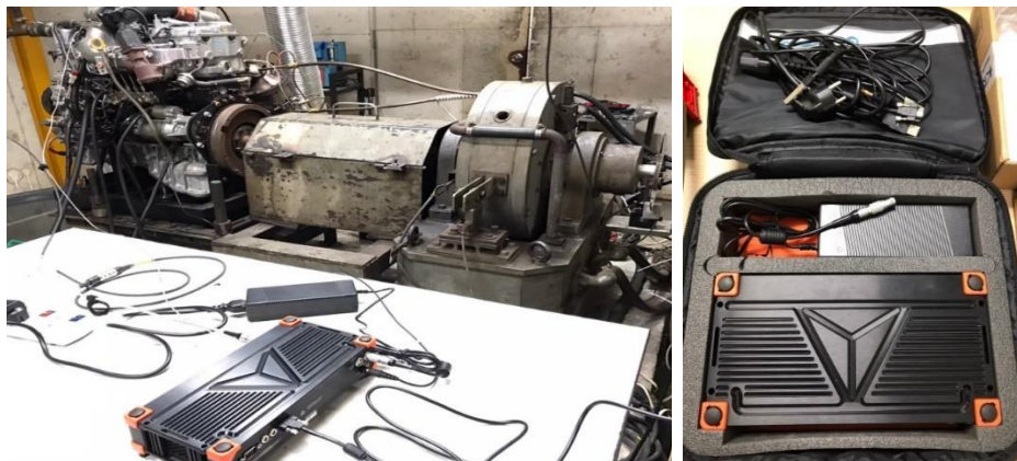
Figure 3-10 Dewesoft Data Acquisition System
