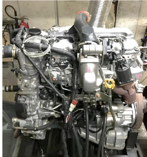
Figure 3-2 ISUZU 4JJ-TC Direct injection diesel engine
