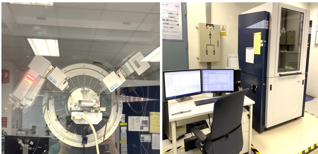
Figure 3-22 X-ray diffraction apparatus employed in this study
