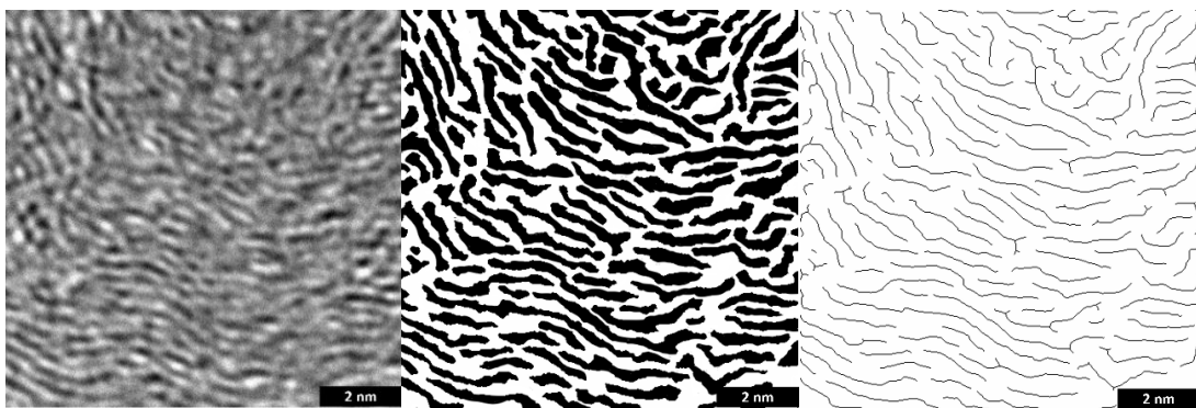
Figure 4-6 ImageJ combined with TEM image analyzing process
