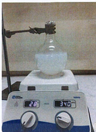
Figure 3.1 Experiment set for synthesis of silica nanoparticles
