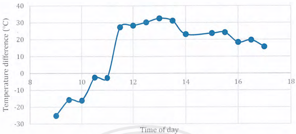
Figure 4.14 The difference between outlet and inlet temperature of propylene glycol at 50 kg/h
