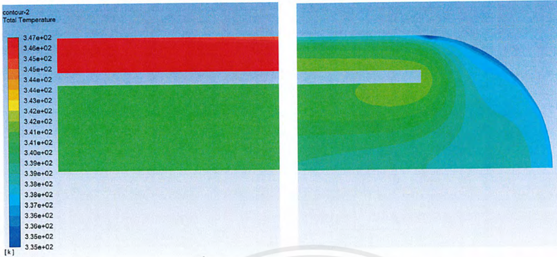
Figure 4.25 Temperature profiles of the design 1 containing stainless steel 403 of outer tube and tube head radius R design
