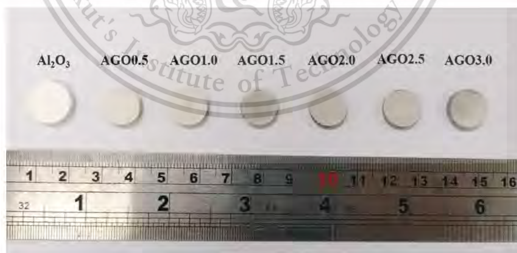
Figure 2. The appearance of pristine \text{Al}_2\text{O}_3 and AGO composites sintered at 1500°C.
