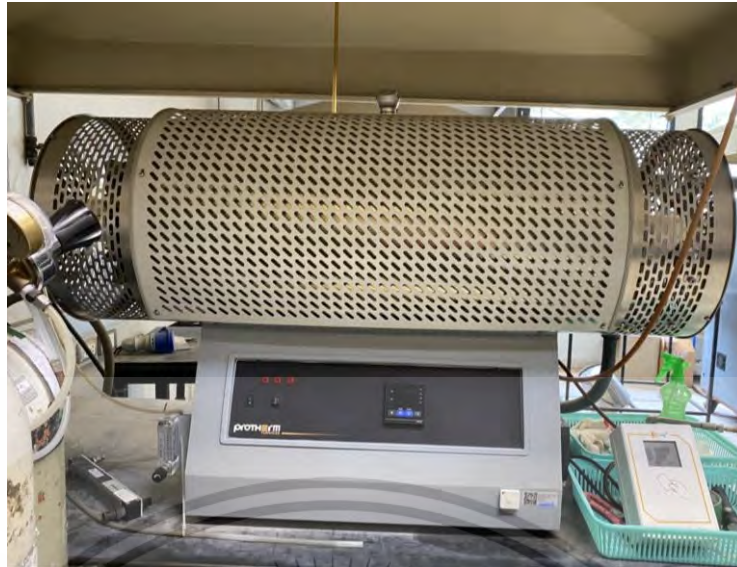
Figure 3.2 Tubular furnace for alumina-carbon composites sintering.
