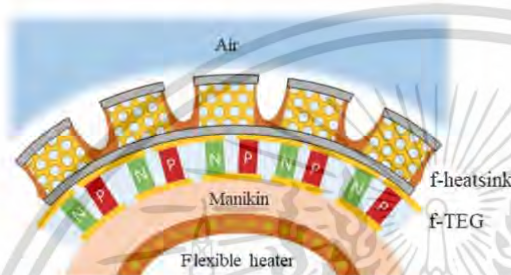
Fig. 4. Schematic diagram of the experimental setting for the V_{oc} measurements.
