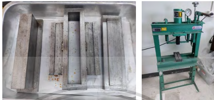
Figure 3.3 (a) Steel mold and (b) hydraulic pressing machine.
