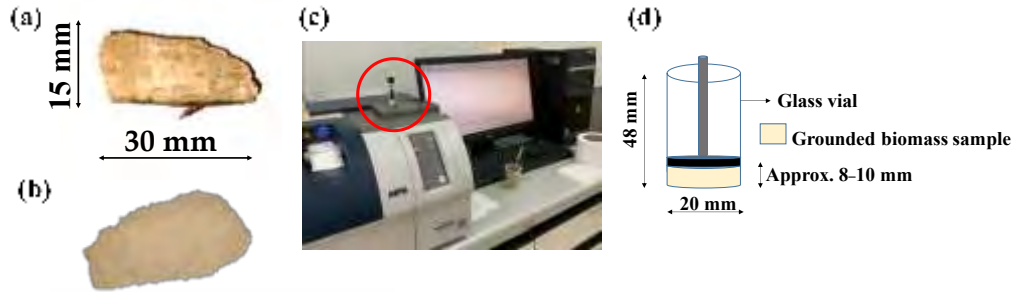
Figure 3.2 Nepal biomass in (a) chips form (>30 mm × 15 mm), (b) grounded form (1.88–3080 μm), (c) FT-NIRS (MPA, Bruker, Ettlingen, Germany) scanning between the wavenumber range 3595 to 12,489 cm -1 , and (d) ground sample presentation by transmittance mode.
