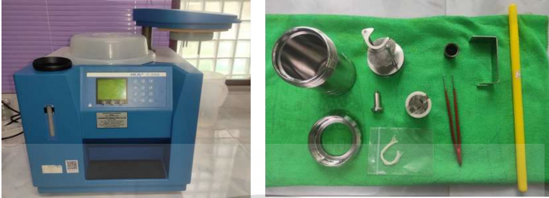
Figure 2.9 Automatic Bomb calorimeter (IKA C 200, Staufen, Baden-Württemberg, Germany)
