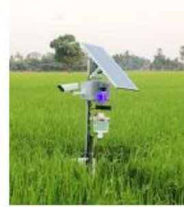
Figure 4. The quantity measurement of pest box imaging machine
