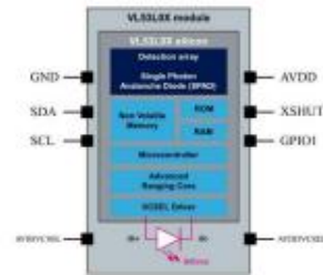
Figure 7. Laser ranging VL53L0X block diagram
