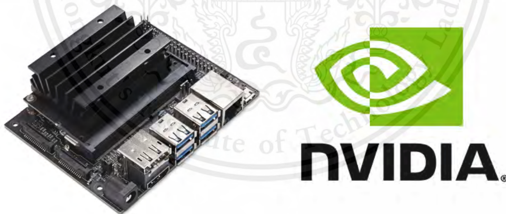
Figure 16. Jetson Nano developer kit [27]
