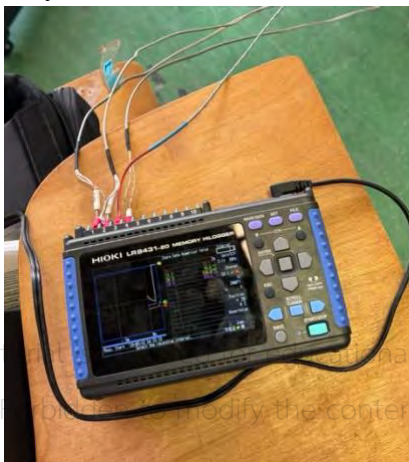
Figure 3.6 : data logger ( MEMORY HiLOGGER LR8431-20 )
